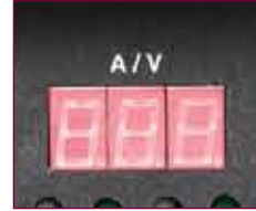
Digital welding/Pilot current amp meter.
